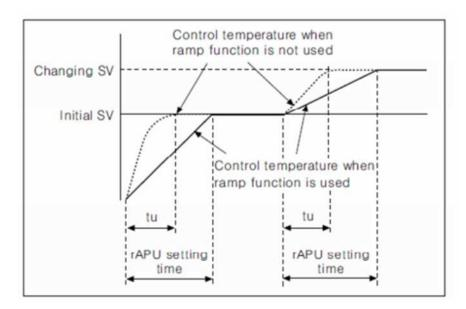
It makes delay rising temperature when change the set value at stable control status or delay the initial rising temperature as like above picture. Note1)rAPu time cannot be set shorter than temperature rising time(tu), when Ramp function is not used.
