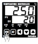
4 Press MD key when the setting is completed. It will stop flickering, then return to RUN mode.
